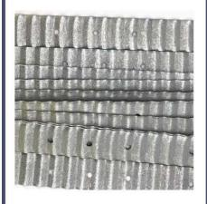
By tweaking the steel composition and switching from hot-dip and spun galvanizing to mechanical galvanizing, we achieved a breakthrough. Our new process ensures a wellbonded, evenly coated, and dust-free surface. The result? A vastly improved product for our customers. streamlined internal packaging, and a better experience for the end user.
