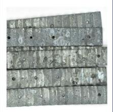
Hand sorting became a necessity to separate the stuck parts, which significantly increased packaging time. During this process, we also discovered another issue: coating powder and dust residue that needed to be cleaned up before packaging.
